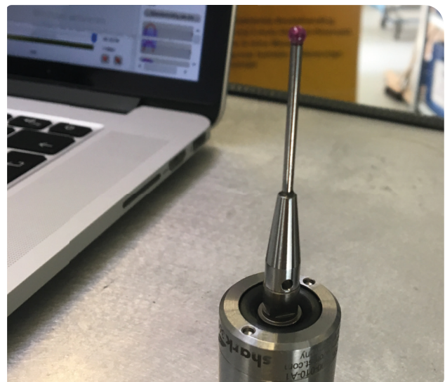
Tactile measuring probe to measure Preface blanks and glass ceramic blanks. The probe is also used for the quality control of outer telescopes and for the determination of possible re-millings.
