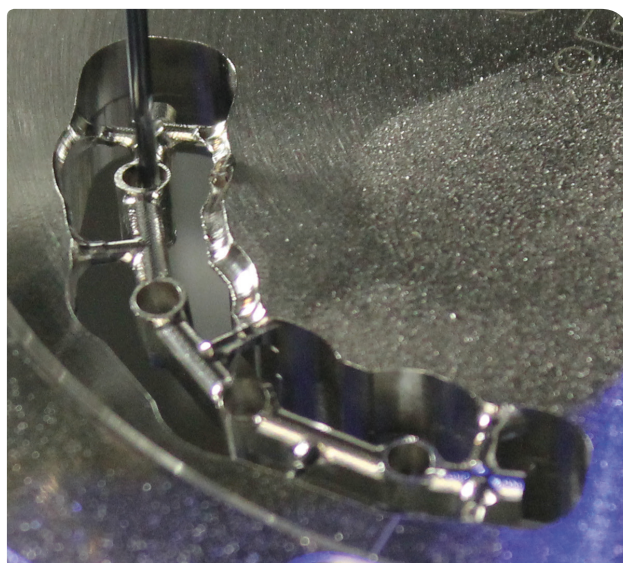
Manufacture your own bars from titanium or non-precious alloy.
